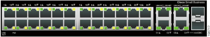
**RJ-45 Ethernet Ports**—Use these ports to connect network devices, such as computers, printers, and access points, to the switch.
